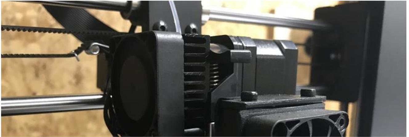
*Example of a spring-loaded direct drive*
